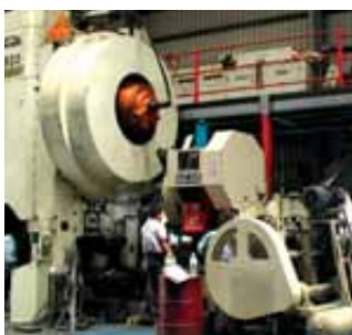
Left: Manufacturing of anchor shackles for offshore application.
