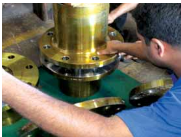
A propeller shaftline undergoing alignment, coupling, contact and bluefit test and class inspection.
