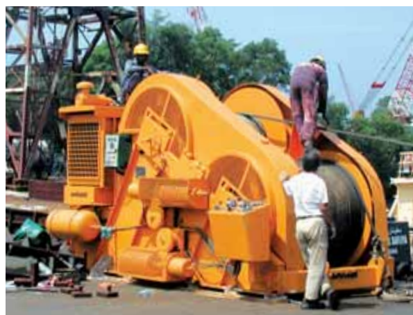
Right: Spooling of wire rope onto the second layer of an offshore winch.
