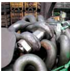
Left: Manufacturing of anchor shackles for offshore application.
